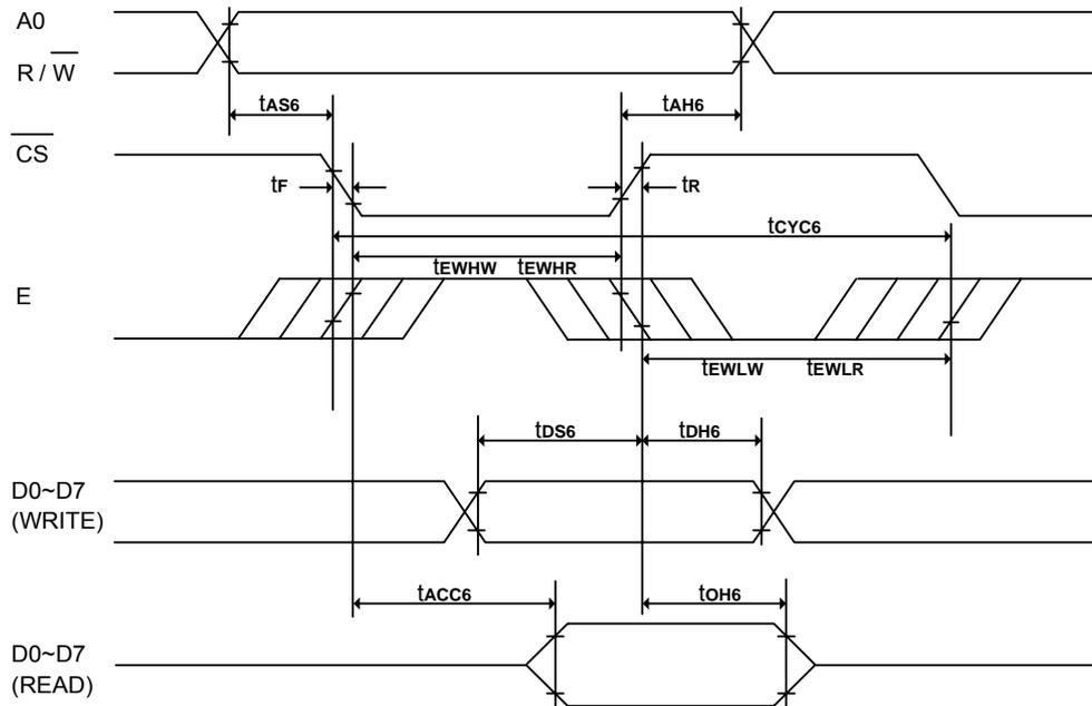
(V<sub>DD1</sub> = 2.4 - 3.5V, T<sub>A</sub> = +25°C)
